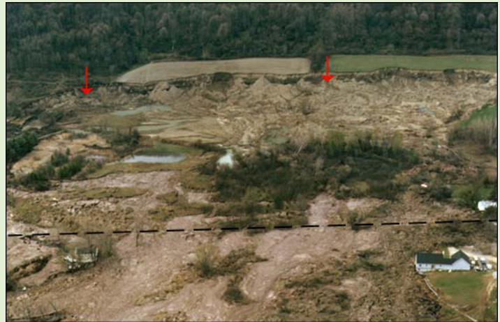
Figure 1: Oblique aerial view of the Tully valley landslide taken April 30, 1993, three days after the slide. Debris moved toward the viewer, in the process covering Tully Farms Road (dashed line) with up to fifteen feet of reddish remolded clay. Three people were rescued by helicopter behind the white house (lower left) from the rapidly advancing landslide. Springs are located between the red arrows.
